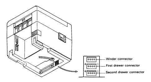
Connector Printer side : 5045-04A (Molex) Cable side : 5209-04 (Molex)
